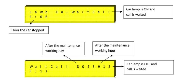
When the car is moving, on the left side of LCD top line, there is target floor and on the right side of LCD top line, there are movement direction, speed and fault datas. On the lower line, the floor that the car position at the moment is screened.
