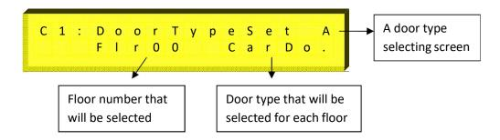
For selection, with lightening left arrow by pressing ENTER button, required floor is selected.
