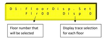
It is used for trace type selection that is required to be traced on floor for every floor. To change the parameter; first, by pressing ENTER button, floor is selected with arrow on left side. By pressing ENTER button again, display that will be traced is adjusted with arrow on right side.
