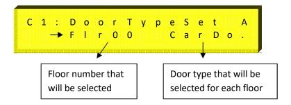
If floor door type is required to change, it is pressed ENTER button second time and lightened right arrow and door type is selected.
