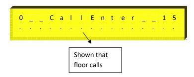
Dots on the screen indicate floor numbers in order. Floor that will be given call is selected with cursor and put "+" sign with "ENTER" on the floor number. More than one call, the other floors are selected the same.
